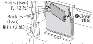
Insert the housing completely to the end. 将外罩切实嵌入到底。
