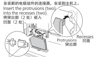
Align with the direction of the line 对准线的方向
