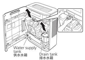
Take it out carefully to avoid water spilling. 请小心取出,注意避免水洒出。
