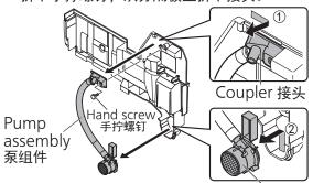
② Lift the drain pump up to pull it out.
