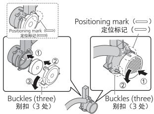
5 Install the pump assembly onto the partition plate.
